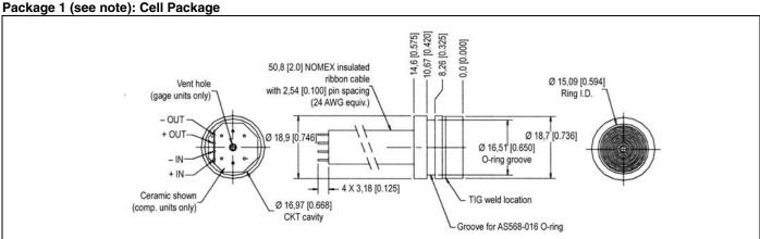
Note: Non-concentricity effects at the diaphragm weld area may cause runout of up to ±0.006 in between the upper and lower portions of the sensor body. (It is recommended to use a counter bore to mate with this device to allow for this non-concentricity).
